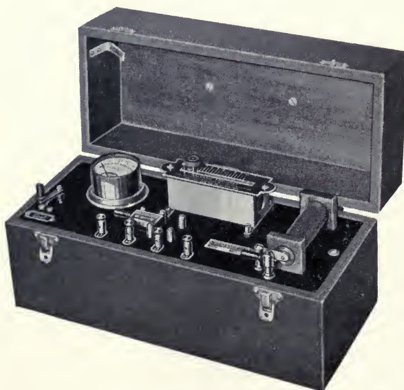
FIG. 125.—Portable galvanic and faradic battery. The galvanic current is supplied by two 45-volt batteries contained in the cabinet. Useful at the bedside and where no lighting current is available. Current output is even while dry cells last.
